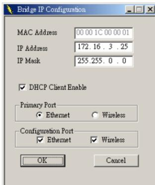
This option enables / disables the DHCP client function of the AP. Additionally you have to select the Primary Port, which is the interface that determines the DHCP server. You can also choose to use either Ethernet and/or Wireless port for the AP configuration.
